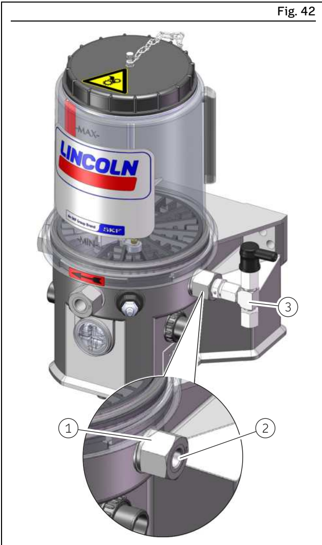
Replacing pump element and pressure limiting valve
