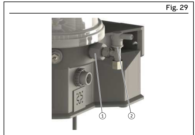
Installing the pressure limiting valve
